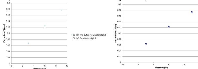
Figure 6. Flux responses for increasing pressures with 50 mM Tris Buffer and DiH<sub>2</sub>O flow material. Flux responses to increasing pressures for 0.2µm membranes with 100%, 40%, and 0% 2-BiB concentration activation (Right). Decreasing pressure measurements were also performed but not present here because the descending results matched the initial pressure values. Measured using a Direct Flow Filtration Unit.
