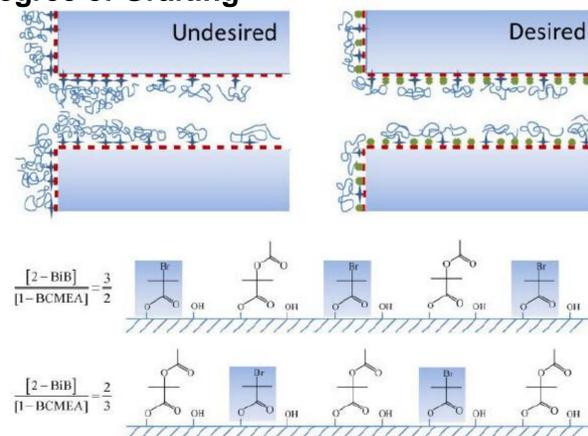
Figure 4<sup>2</sup>. Non-uniform and uniform distribution of initiator molecules (top left to right respectively). Localized densities has the potential for pore constriction. Initiator is spaced throughout the membrane pores using a non-ATRP-active molecule, in this case 1-bromocarbonyl-1-methylethyl acetate (1-BCMEA). The initiator used was 2-bromoisobutyl bromide (2-BiB). Initiator grafting density was varied by altering the concentration ratio of 2-BiB/1-BCMEA in solution.
