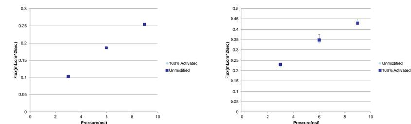
Figure 7. Flux responses to increasing and decreasing pressure 0.45µm (Left) and 1.0µm (Right) membranes with 100% and 0% 2-BiB concentration activation. Decreasing pressure measurements were also performed but not present here because the descending results matched the initial pressure values. Measured using a Direct Flow Filtration Unit.
