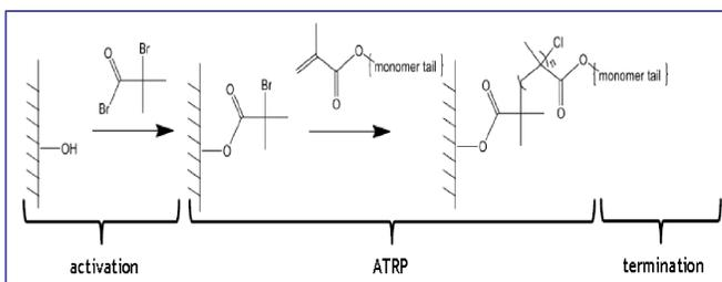
Figure 2. Two-step modification procedure. Initiator molecules were attached to the membrane pore surface in the first step. Atom transfer radical polymerization (ATRP) was used in the second step to graft chains from the initiator sites.
