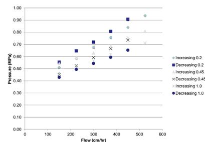
Figure 5. Pressure responses to increasing and decreasing flow for 0.2µm, 0.45µm, and 1.0µm unmodified membranes. Measured using an Äkta purifier machine.
