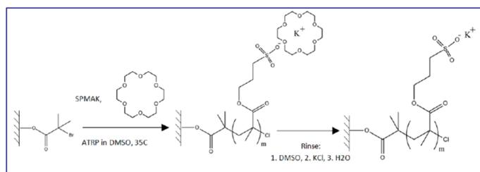
Figure 3<sup>4</sup>. ATRP reaction scheme. The crown ether is used to facilitate monomer dissolution and reduces undesired side reactions. Ascorbic acid is added to the ATRP system to act as a reducing agent that quickly converts any oxidized Cu(II) to Cu(I).
